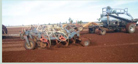
Plate 3.2 The airseeder, fitted with presswheels, is used for all sowing at 'Hill End'.
