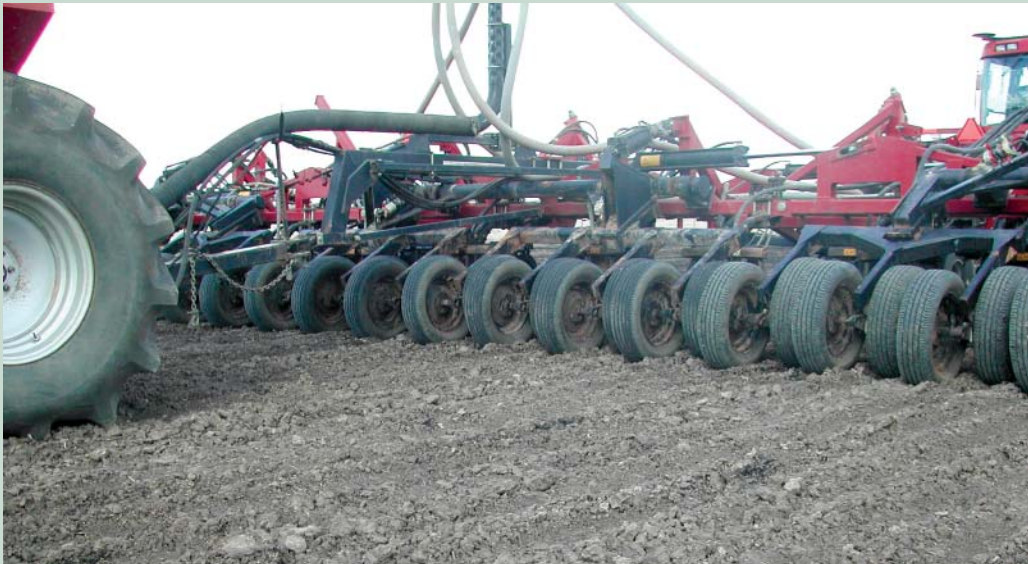
Plate 2.3 The press-wheels of the Concord 4812 produce a corrugated surface which assists in water harvesting for the emerging crop.
