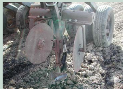
Plate 2.2 The coulter, tyne and press wheel configuration of the Case Concord 4812.
