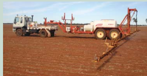
Plate 3.1 The Hino 4x4 gooseneck boom spray used at 'Hill End'.
