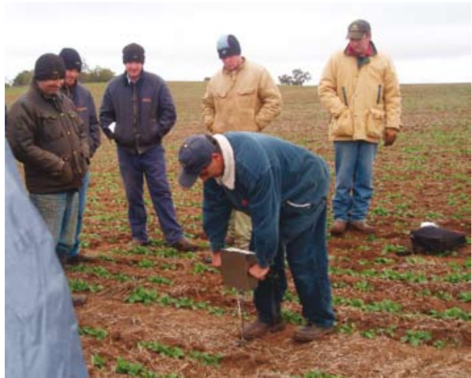
Measuring soil strength using a penetrometer at the Bobbara Station Field Day 2007.
