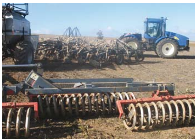
Terry Brown's Flexicoil air seeder with tow-behind air cart and coil packer.
